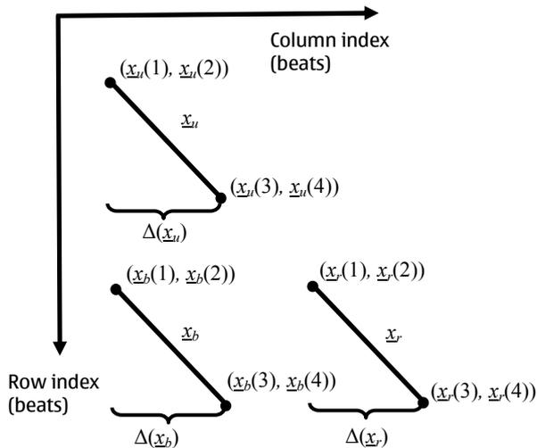
Figure 5: Notations when giving scores to a group of three diagonal segments (detected stripes of small distance of the distance matrix). The units are measured in beats.
