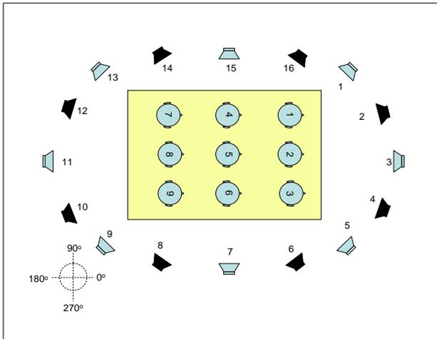
Figure 2: Geometry of loudspeaker array and audience area for monophonic listening tests.
