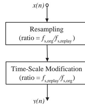
Figure 1: Block diagram of the pitch-shifting method based on the resampling and time-scale modification.
