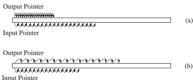
Figure 2: Effect of resampling process on the speed of the output pointer, (a) signal is pitch-shifted down, the output pointer moves slower than the input pointer, (b) signal is pitch-shifted up, the output pointer moves faster than the input pointer.
