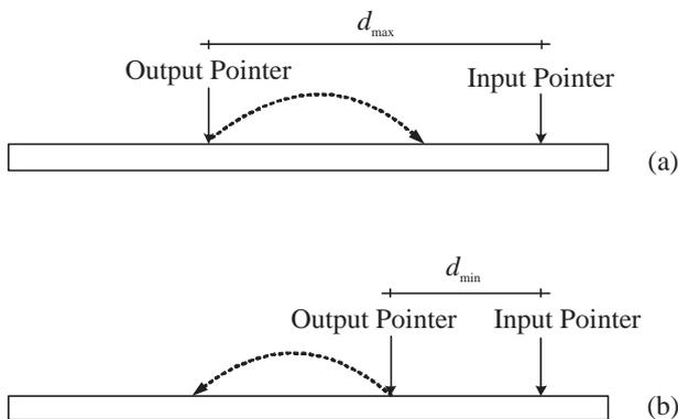
Figure 3: Behavior of the output pointer with respect to its distance from the input pointer,  $d$ , (a) when  $d > d_{max}$ , the output pointer jumps forward, (b) when  $d < d_{min}$ , the output pointer jumps backward.
