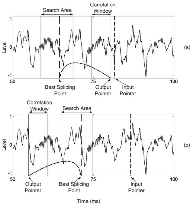
Figure 5: Choice of the correlation window and search area in the search for the best splicing point, (a) the output pointer jumps backward, (b) the output pointer jumps forward.
