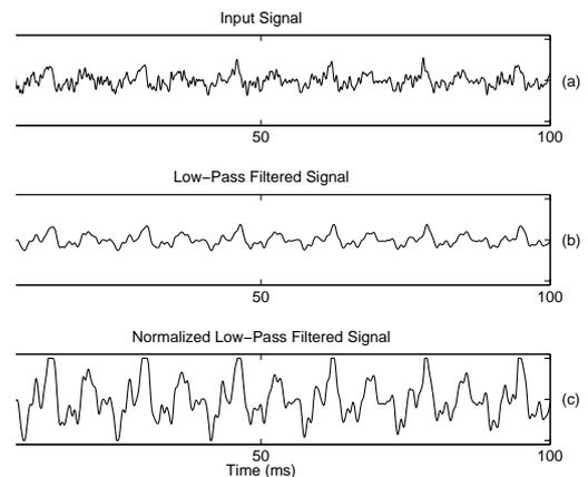
Figure 4: (a) Original signal, (b) low-pass filtered version of the original signal, (c) normalized low-pass filtered version of the original signal.
