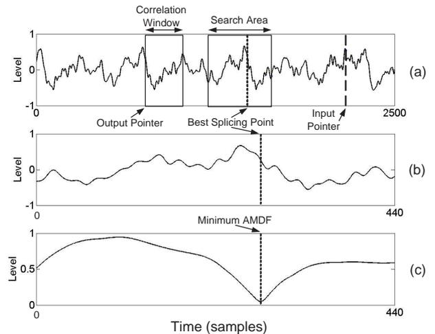
Figure 6: Search for the best splicing point, (a) part of the ring buffer in which the correlation window and search area are placed, (b) the search area in which the best splicing point is looked for, (c) the AMDF over the search area for the shown correlation window.
