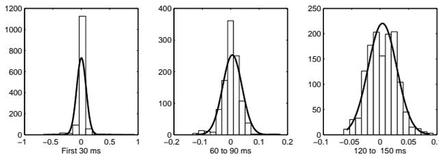
Figure 2: Progression in time of histograms and fit normal functions of 30 ms windows of an IR. Note the differing vertical and horizontal scales. The absolute values of the vertical scale are not important, but rather the relative values between the histogram bars. The range of the horizontal scale decreases in subsequent windows because the signal is decreasing in amplitude. It is important to note the distribution of the samples, not the absolute values.
