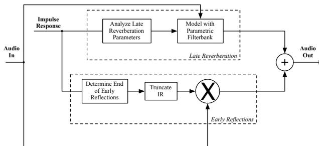
Figure 1: Basic design of a hybrid reverberator.
